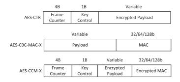
Fig. 3. Payload data formats with IEEE 802.15.4 security.
