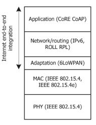
Fig. 1. Communication protocols in the IoT.
