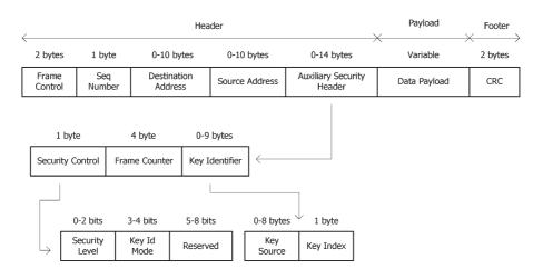
Fig. 2. Security data and control fields in IEEE 802.15.4.
